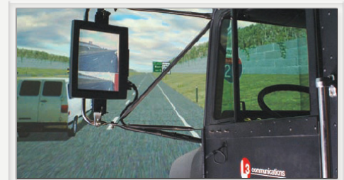
Two LCD screens simulate the rear view from the truck cab
