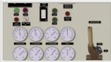
Interactive virtual local controls and instrumentation for a Medium Speed Marine Engine.
